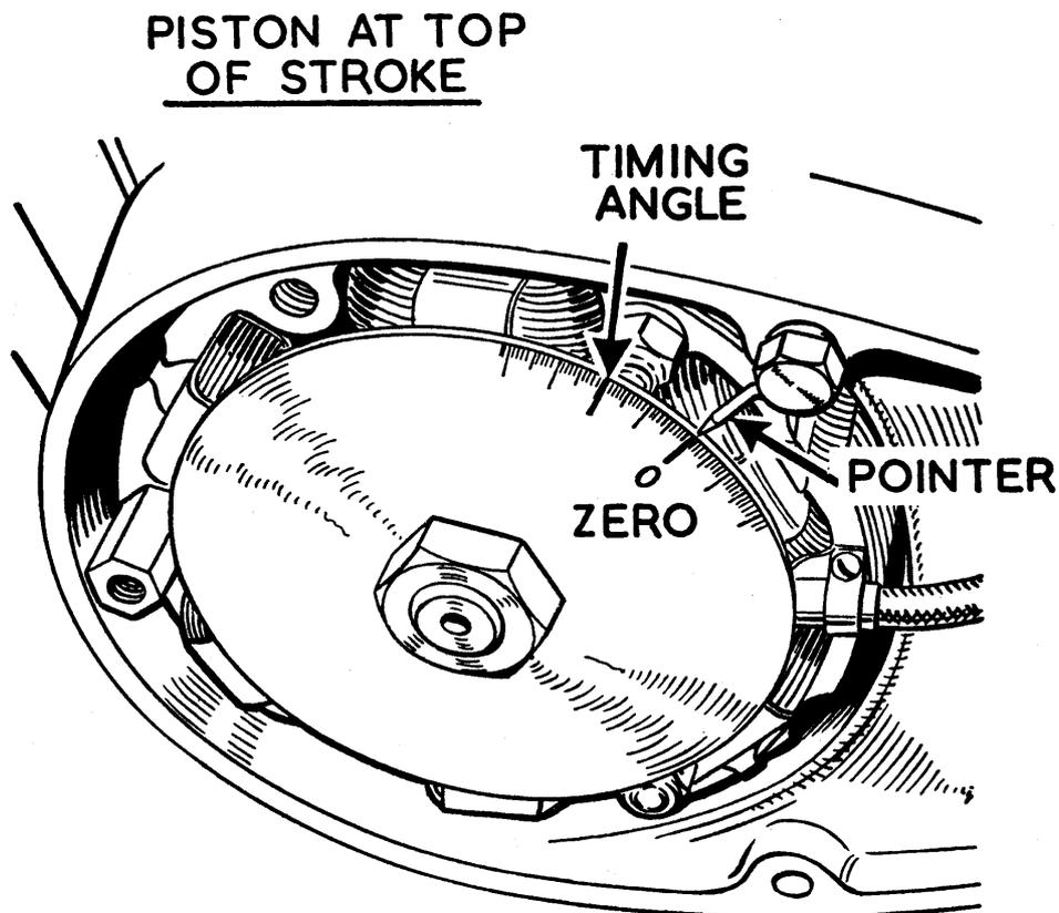
Fig. 3. Timing the engine with a degree plate
