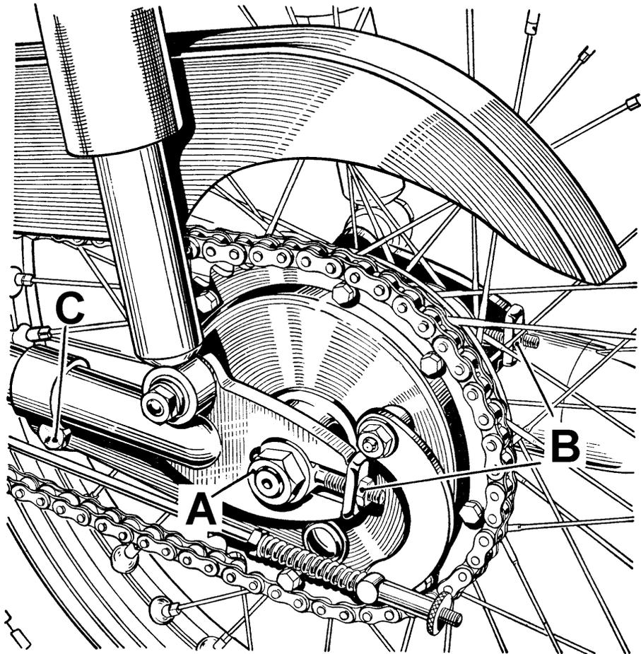
*Fig. 8. Rear Chain Adjustment*
