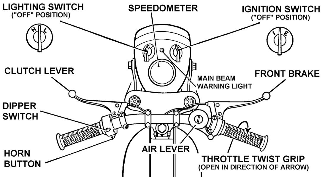
*The controls of the Bantam Sports. Note: Bushman models are not fitted with an ignition switch, main beam warning light, or parking light, but are otherwise similar.*
